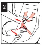
Loosen harness by pushing down on the harness release lever while pulling out on the harness.
